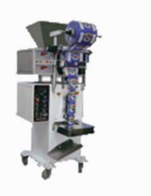
This series packing machines also produce pillow-shaped package sack but use electric weight method. They are suitable for packing loose and a tactic shape material such as tea, expanded food etc. These machines can automatically complete weighing, feed, making sack: sealing, cutting and transportation.
