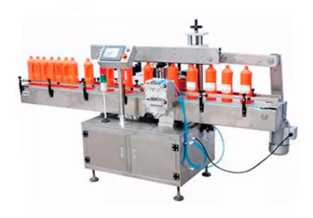
This machine is used for the surface labeling of the round, square and flat objects in such industries as medicine, daily chemical, food, and cultural supplies and so on. It can paste three labels at a time. One label is on the front, one label is on the back, another label in on the top
