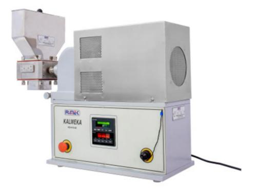
Dry Granulator is used to granulate tablet slugs and pellets. Two power drive rollers with teeth force material against breaking combs. Special design results in low proportion of power. When using hard slugs, from 2 to 2.5 mm thick, the following granulation will be obtained, 45% - 16 mesh, 25% -24 mesh, 10% - 70 mesh, 20% powder. The dry granulator is suitable for screwing on all main drive units.
