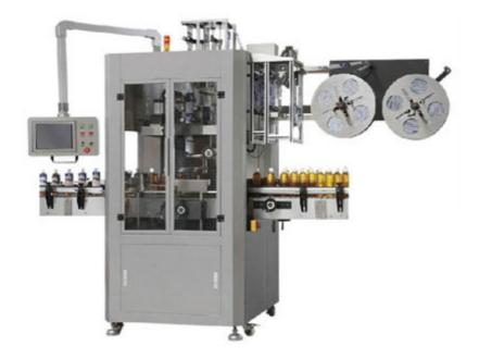
Automatic Sleeving Machines MT-350 adopts PLC programmable controller, imported servo motor, servo driver, frequency converter and transducer; besides, it adopts the positioning module to ensure the casting label precise, rapid and stable. It not only has a highly precise position for casting label, but also can withstand the perfect shape of the bottle after shrinkage.
