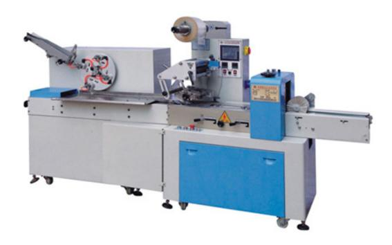
It is applied to feed automatically for cards, mote and patches, which can be customized long card suckers, suitable for packaging multiple cards
