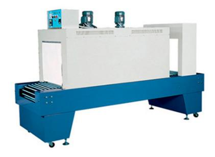
PE Shrink tunnel is equipped with fully re-circulating air chamber and discharge end cooling fans. This shrink tunnels are designed in stainless steel with the 1/4 HP blower motors, heating circulating type, silicon fiber tube on the conveyor rods and dead roller conveyor system for all types of shrinkable films. Like other shrink tunnels, this also can be integrated with L-Sealer machines or overwrapping machines for wrapping improvement.
