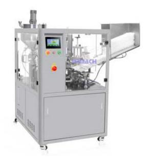
Ultrasonic tube filling and sealing machine uses intelligent digital ultrasonic technology to enable molecules on the surface area of the tubes to be fused together by ultrasonic friction. Intelligent digital ultrasonic welding avoids the disadvantages that weak welding causes due to foreign matter adhering to the walls.
