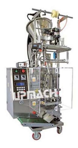
Powder Sachet Packaging Machine is used for sachet packaging of power, such as milk powder, drinking powder, medicine and chemicals powder, starch, pesticide, veterinary medicine, premix, additive, condiment, feed, enzyme preparation and other powdery products. DXDF series sachet powder packing machines are widely used in pharmaceutical, chemical, foodstuff and other industries.
