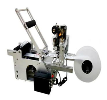
Suitable for different size of adhesive label or adhesive film on all kinds of round bottle, High accuracy and high speed, dispensing & labeling automatically.
