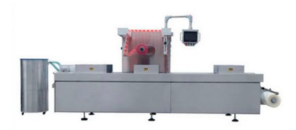
HVR-A model has been designed to pack food and medical products, capable of both flexible and rigid packaging.
