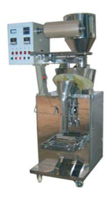
All the works of bag making, measuring, filling, sealing, cutting, counting and heat printing codes can be done automatically, It is adjustable and shake extent of counting table plate.
