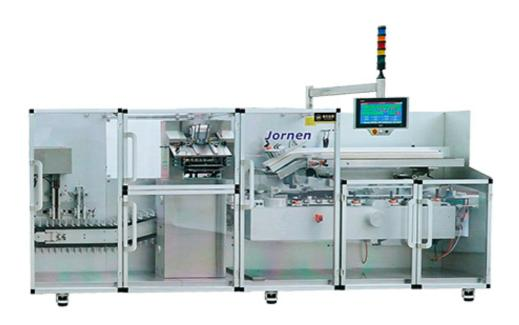
ZH500 is the fastest Continuous Motion Cartoning Machine in our company. It is suitable for pharmaceuticals, food, household chemicals, hardware, and electrical industries for the packaging of blisters, bottles, vials, pillow packs, toothpaste, etc. It can fold leaflets, open cartons, insert the products and leaflets into cartons, emboss, tuck-in, or hot-melt closures and automatically discharge cartons.
