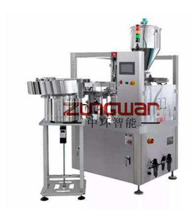
Compact design, tube load by hand, and driving part fully closed. The whole process of filling, folding (heating), sealing, printing, cutting, and finished products output all finished automatically.
