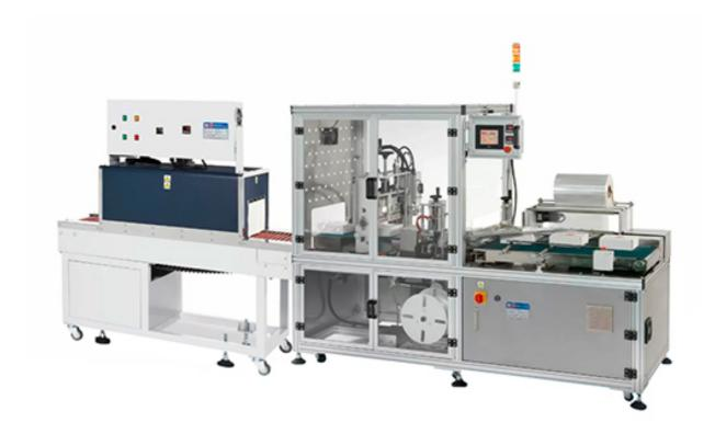
Auto Side Sealing Machine, standard model USA-004BR(CE) can adjust its packaging height basing on product to have strong seal & nice look. USA-004BR(CE) adopted constant heating sealing knife by SSR control to keep stable temperature, power saving and easy change. POF is recommended to work with. USA-004BR(CE) can reduce the film wastage & seal multiple length without any limitation. Simple design, easy operation, film saving & high efficiency, it is the latest model of wrapping machine.
