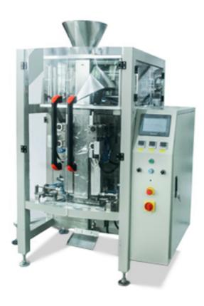
Quad seal bag / block bottom pouch packing machine is suitable for automatic packaging various kinds of leavened food, candies, peanuts, seeds and such materials in grain or piece as well as powder like milk powder, washing powder, starch, etc.
