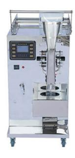
Liquid packaging machine is widely used for packaging liquids such as purified water, milk, fruit juices, beverages, vinegar, chili oil and wine. It automatically packing, prints a date code, fills the product accurately and seals and cuts in one go.
