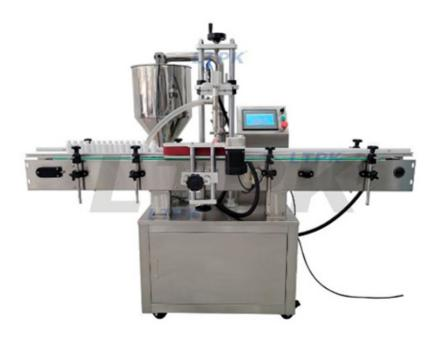
The automatic single head rotor pump filling machine is controlled by a PLC touch screen control panel. Servo motor control, stable and fault free, equipped with automatic feeding function. It has the characteristics of long service life, easy maintenance, stability and reliability, convenient operation, accurate measurement, and fast speed. Heating and mixing function can be customized as production need.
