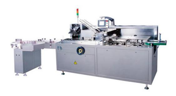
Automatic Box Packing Machine is suitable for inserting blisters, bottles, vials, tube, ointment, sachets, injections, cosmetic, condom, ampoules, plow-wrapped products, soap components, automotive parts, hardware, frozen food, milk powder bag, cereal bag, pharmaceutical products into carton in a range. It is high technology product incorporates of pneumatic-photo-electromechanic.
