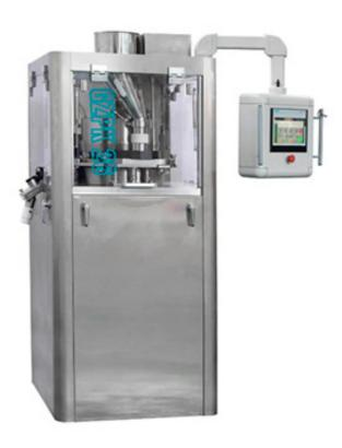
This high-speed rotary tablet press machine offers the capability to produce a large volume of round and special-shaped tablets. With its double pressure structure and 33 die sets, it can efficiently press up to 66 tablets in one rotation while allowing adjustments for speed, filling depth, and tablet thickness. Equipped with a powder suction box and mechanical buffer device, this machine ensures smooth operation and high-quality, dust-free tablets in line with GMP specifications.
