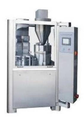
SPR-8 Automatic Capsule Filling Machine. Small volume, low consumption of energy, simplification in changing modules. Easy operating and cleaning. Adopt eliminating Ma's trough roller to transmit, less vibration, its noise is lower than 75dB while running at top speed. Dose difference is controlled within ±3%. The rate of capsule filling is>99%.
