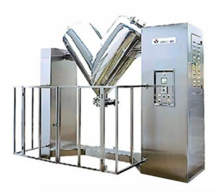
V-Mixer is suitable for the powder, granule, lubricant adding, binder, seasoning's adding and mixing of western medicine, Chinese medicine and health food. Its unique V-shape design makes the raw materials mix together quickly and evenly during the mixing process, and the inner part of the machine is easy to clean, which is suitable for mixing many different types of raw materials.
