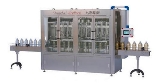
The automatic edible oil filling machine is specially designed for oil filling. The technical details of each machine are based on the characteristics of different edible oils. It adopts the design of a back-suction nozzle to ensure that there is no leakage problem. The servo motor drives the piston, filling accurate and stable.
