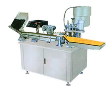
This SD-YGF-55 liquid filling sealing machine (oral filler sealer) is a kind of specially designed packaging equipment that is used for the filling and closing-over of oral-taken liquid. It is composed of auto-bottle-in, filling, fixing lid inside, closing-over and bottle-out. It can be equipped with a creep-age pump to meet different needs. Also this machine can be controlled by a mini computer.
