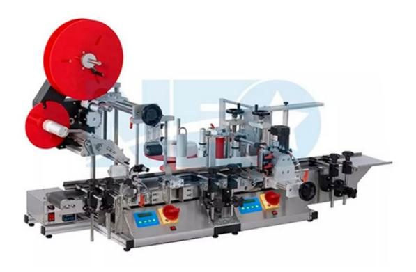
Equipped with a round bottle labeling head and a top labeling head, wrap around and top labeling LR1300 and LT1100 tabletop labeler fulfills labeling tasks of round bottles and top label through one single process. Its greatest advantage is its capacity of carrying out the two labeling tasks within one single process.
