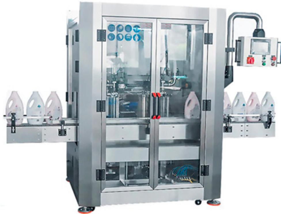
Introducing our revolutionary Automatic Tracking Filling Machine, a game-changer for your business! This cutting-edge machine is designed to streamline your bottling process, allowing for seamless filling without the need to pause or stop the bottles. Equipped with advanced servo motor control and four filling heads, it has the capacity to achieve an impressive speed of up to 5000 bottles per hour.
