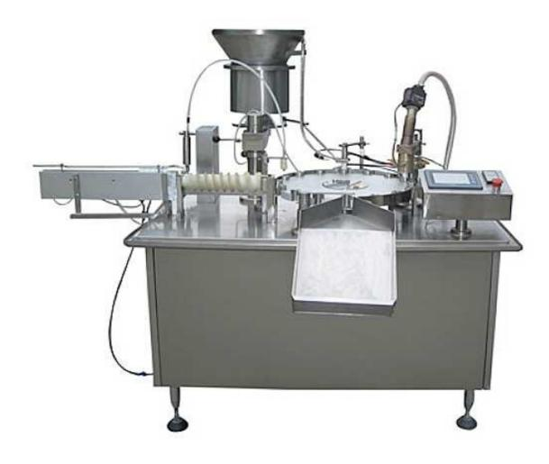
This machine is suitable for filling and sealing to easy-folding plastic bottle. Automatic feeding, filling the bottom, hot-melt sealing. PLC control, touch screen operation; missing bottle, no filling; automatic counting, functions steady.
