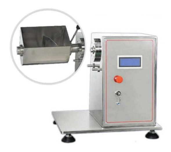
DGN-2 Main Machine + Trough Type Mixer. Trough mixer adopts a Z-chip to rotate in the groove container in different angles. It is made of stainless steel, with the different speed and the outline of stainless chip, it mixes materials very well. The whole container can rotate at a 180 degree after cutting off the power, so it is easy to discharge and to be cleaned.
