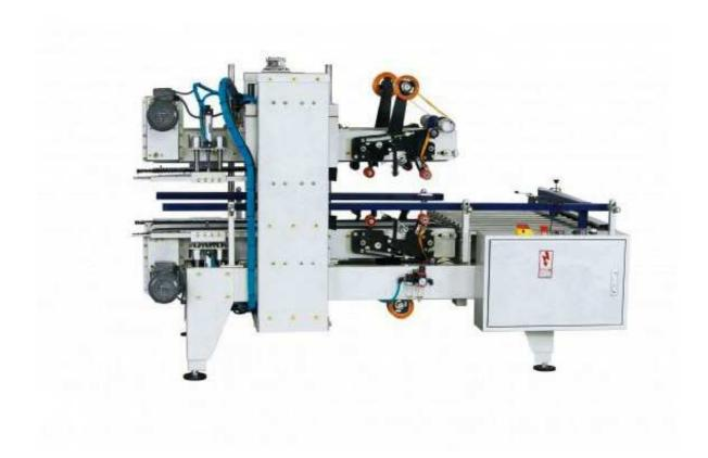
Carton sealers are case equipment that seals the top or bottom of a case with tape or glue. Typically, the minor corrugated flaps are kicked and plowed closed as the cases are transferred. As the cases enter the compression section, the major flaps of the carton are closed and a hotmelt adhesive is applied.
