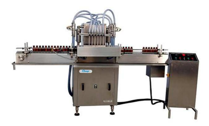
Automatic Volumetric Liquid Vial Filling Machine work on volumetric principle with diving nozzles. The unit is made compact, versatile and enclosed in stainless steel elegantly matt finish body, consists of S.S. Slat Conveyor, Reciprocating Nozzle with self-centering devices & SS Syringe. No container No filling system arrangement is standard features of the machine.
