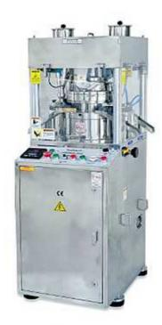
Lab Press – SDL-2 is a High Tech Double Layer Rotary Tablet Press for R&D and small batch production. This Single sided R & D Double Layer Tablet Press fully conforms to GMP and the safety requirements. The Turret is driven centrally by a motor and Reduction gear box. The turret speed is adjusted by A.C. frequency drive. Its available in Regular Model D' Tooling or B' Tooling Multi Tooling – D+B Tooling or D+B+BB.
