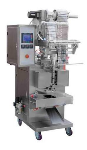
The machine can automatically all processes, including bagging ,measuring, filling, printing the date, cutting and counting, suitable to measure and package powder, material with different fluid characteristics such as milk powder, coffee, washing powder, dye, essence, flavors.
