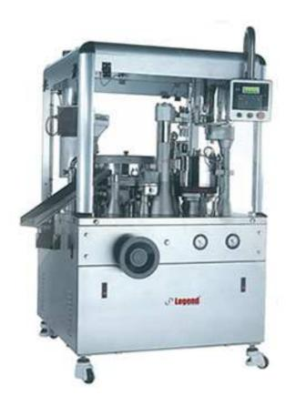
Encapsulation is the filling of empty capsule with the desired drug. It is done using tamping principle. In this the powder formulation is formed into a slug, which is delivered to the body of capsules. This machine can fill hard gelatin capsules with powder, granules, and pellets.
