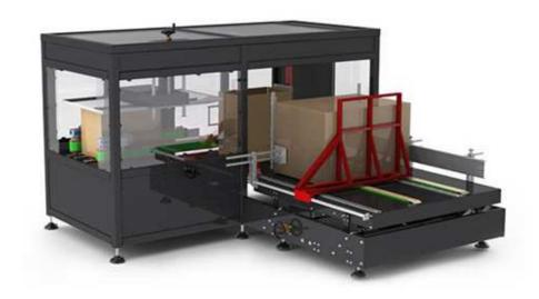
The BEM300 Automatic Case Former is an automatic case forming machine from Spanish manufacturer Ear-Flap with manual size adjustment, PLC control and capable of forming up to 8 cartons per minute.
