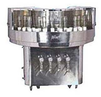
VEENA PHARMA MACHINERY rotary bottle washer is compact, highly efficient and elegant in look. It has many functional features as per GMP standard to wash containers of glass, plastic or other material. The machine operates on the rotary principle with GENEVA mechanism and requires manually loading and unloading of bottle
