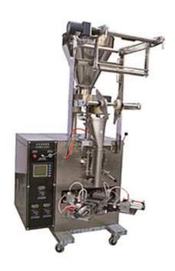
The machine is suitable for packing non sticky, bulk or granular material, such as medical pills, tea, food Stuffs, plant seeds, washing powder, coffee, sugar, desiccant etc The integrated processes of bag making, measuring filling, sealing cutting, counting and hot pressing codes can be done automatically. Packing material includes several kinds of heat seal lamination, such as PET/plated AL/PE, PET/PE, PAPER/PE, NYLON etc.
