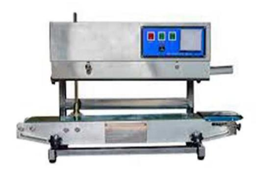
The machine adopts electronic constant temperature mechanism and steeples speed adjusting transmission mechanism. It can seal plastic films with various of materials. such as PP, PE, Alumlnum foil, laminated material. And can fixed date embossing system, If necessary, counting device can be fixed to the machine.
