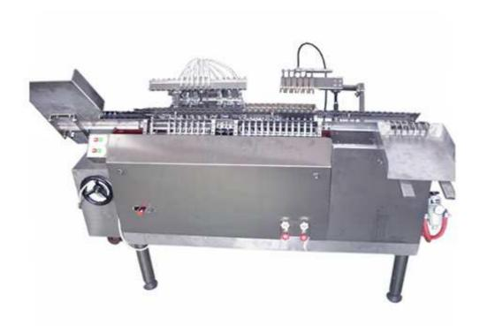
Filling and sealing machine for ampoule Model SLAG-6A is equipment specifilized in filling and sealing 5ml to10ml, and 15-20ml bottle in pharmaceutical works. This machine is equipped with automatic stop-filling device which can make filling case when there is no ampoule into filling station.
