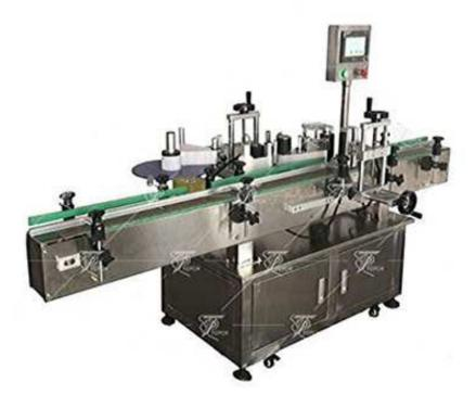
Automatic sticker machine, vial labeling machine, bottle labeling machine widely used for different sizes of round products such as round bottles, cans, jars, cylinder in daily chemicals, food, beverages, medicine and other industries.
