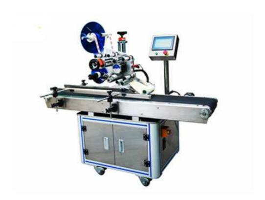
MT-220 model plane non-dry tape marking machine to achieve rationalization of production target and design. Labeling process automation, simple operation, the production speed is quick, labeling position, beautiful, neat, This equipment is mainly used in food, beverage, pharmaceutical, cosmetic, chemical industry, the bottle of single side or plane.
