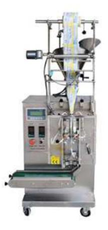
F100 Automatic Three Edge Small Sachet Sealing Packing Machine is specially designed for powder material auto-weighing filling and bag forming sealing. Widely applied in the market of chemical powder, food powder, additives, this machine unit has been accepted by customers for long time.
