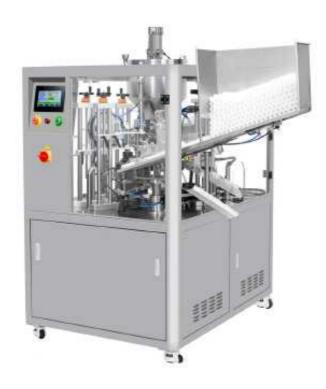
Packry's HX-009 Automatic Cream Tube Filling Machine is suitable for filling all kinds of semiviscous and viscous products into the designated tubes. The tubes will be internally heated by ultrasonic energy and can be coded with an optional date and lot number coder.
