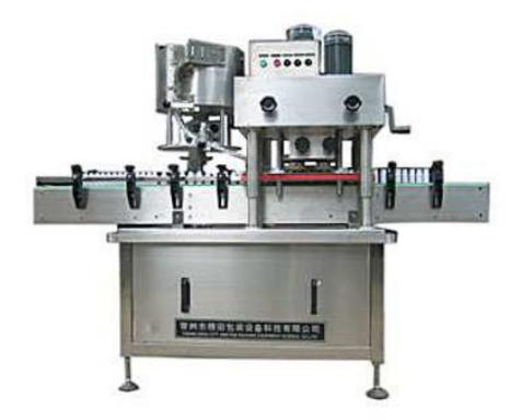
In-line screw cap machine is a new generation of products we introduced and developed, what is widely used in pharmaceutical, chemical, food, beverage, oil and pesticides for automatic rotary sealing, in the production line. It can also configure transport aircraft alone. Its most prominent feature is that it can adapt to all shapes and types of bottle just by adjusting without any additional parts. It is equipped with international advanced Li cover equipment and of high production efficiency.
