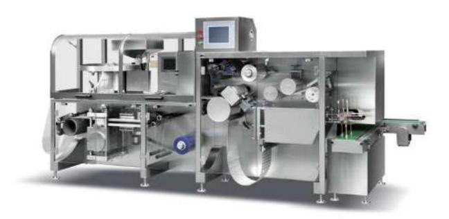
This series machine is at high precise and the latest roller and plate type blister packing machine, developed by our company. it applies to pharmaceutical industry, food industry, medical appliance and electronical area. It is suitable for packing capsules, tablets, milk pieces, candy, electronically element and similar material, with sealing packing in al-pvc, paper-pvc
