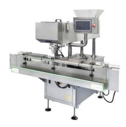
This machine is a intelligent automatic counting and filling machine, which is widely applied for capsule counting for big scale production in hospital, pharmaceutical factory etc. The machine can count & fill different shapes or size of products accurately like soft gel capsules, hard capsules, tablets, sugar coating, and film coating tablets, pills, herb medicine or similar products into containers or vials.
