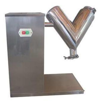
Lab Series V Type Mixer is primarily used in Laboratory for mixing dry powder, granulate or crystal products in Chemical, Food, Pharmaceutical and other industries. By rotating the V shaped vessel, the materials move in convective motion to get a quick and homogenous blending.
