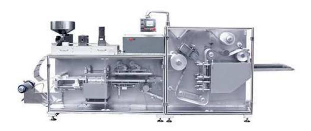
It adopts with flat-plate forming mould, normal pressure to form, blister with homogenous hardness, Roll mash sealing, and is equipped with dot printed, indentation device, cross punching without wasting material, with high automation, high efficiency. It is widely used in pack Alu-PVC package for capsule, tablet in pharmaceutical industry.
