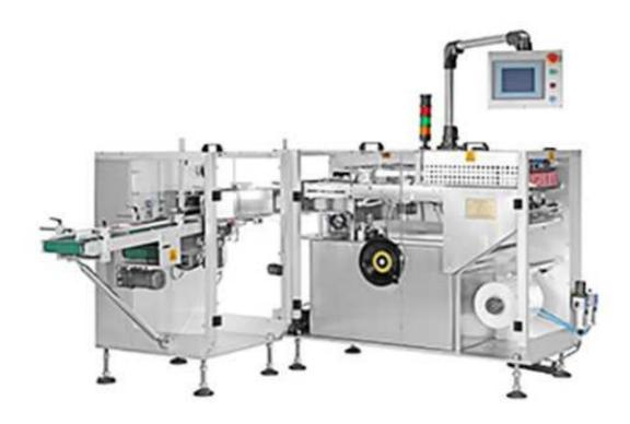
BZ25 film packing machine can automatically complete the function of transport, arrangement, stacking, and then use the material called BOPP for strapping. The very two sides is heat welding to make it a stable strapping. This machine is widely used in pharmaceutical, food, daily chemical and other industries.
