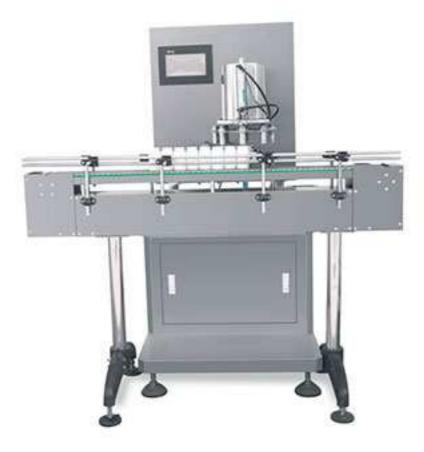
Wide applicability, used for round, square flat and special shape bottle made of plastic. Selfdiagnose and stop working to make alarm at errors and missing bottles as well as change cotton sliver. Patented cotton-insert technology, using pneumatic cotton-insert technology to avoid pollution of materials.
