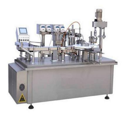
This machine is suitable for filling the liquid in slender cap spray can which is applied in the medicine and cosmetics industries. It performs the whole automatic process including filling, cap placing and cap screwing Special used for pump cap with long tube, with manipulator and guiding device to accurate positioning the pump cap. This machine conforms to the requirements of GMP.
