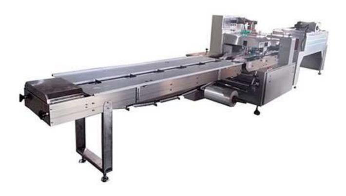
It works from feeding, bag forming to sealing and shrink wrapping, widely used in food, medical, cosmetic and stationery industry.
